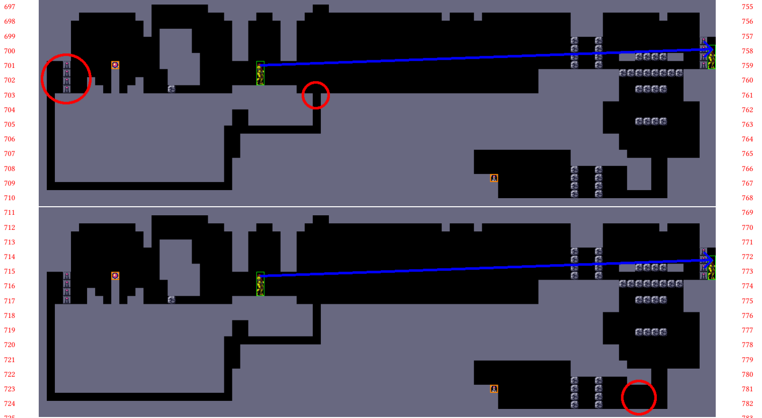
Figure 4: Two modified abstract levels (a) and (b) based on the real level shown in Figure 3. The path on the left (entrances circled) has been added to illustrate how the system detects softlocks. In each level, the blue arrow points from the start state to the goal state. Design (b) is identical to (a) except where circled. Design (a) satisfies AG(EF(goal)) , while design (b) does not. Figure 5 shows why (b) fails this verification. The two item upgrades (missiles and morph ball) are highlighted in orange.
