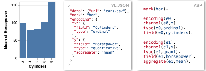
Fig. 2. An example of a bar chart, its Vega-Lite specification (in Vega-Lite JSON), and its equivalent specification using Draco constraints (in ASP). The specification defines the marktype and encodings, which includes a specification of the fields, data type, and data transformations.
